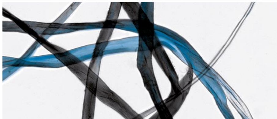
A denim fiber in transmitted-light and fluorescence reveals the typical intermittent effect of the indigo dye
